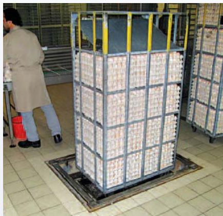
A hydraulic lift set in the floor ensures that all eggs are at an easy level for the hatchery staff to process.
