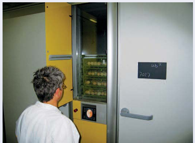
The new generation of Pas Reform SmartHatch hatchers with their new control panels and inspection window.
