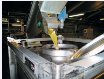
Left, removing non-fertiles at transfer and, right, they are immediately converted to liquid product which is removed in large stainless steel vats.
