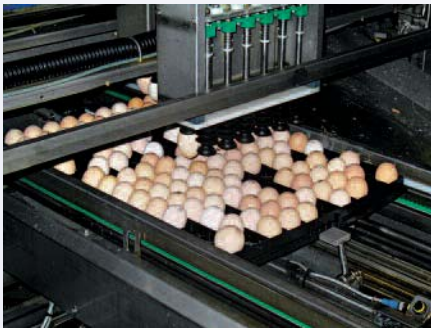
Left, removing non-fertiles at transfer and, right, they are immediately converted to liquid product which is removed in large stainless steel vats.
