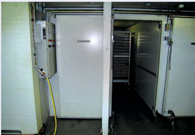
The eggs are fumigated in these cabinets prior to setting.
