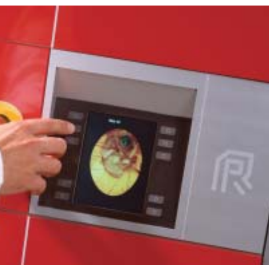
The SmartDrive incubator control system allows careful management of individual conditions per egg type. Features include a pre-heat function, new PID control combined with temperature set points per section and fully adjustable turning programs.
