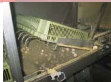
The tray tipper empties a hatcher basket by turning it 180 ° and tipping its contents
