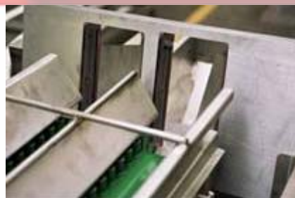
Counting is done as the chicks pass under an infra-red counting head
