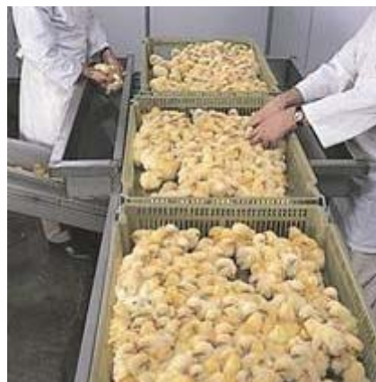
The chick belt of the Pas Reform chick take-off system is placed partly under a non-driven roller conveyor for hatcher trays to give space to four operatives
