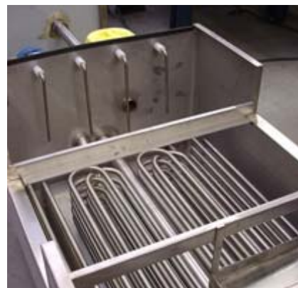
Heat exchanger, which can be used to heat the tank with (indirect) steam or hot water from a central heating system (optional)
